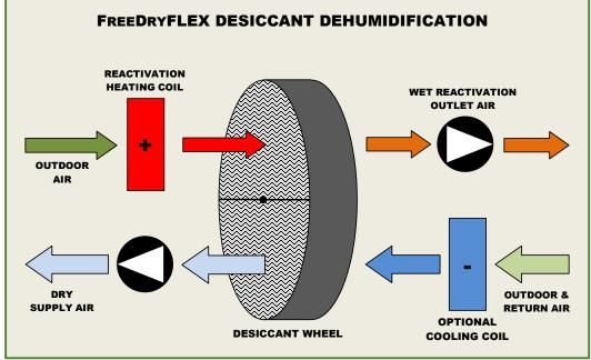
FreeDryFlex<sup>™</sup> dehumidifiers are typically designed to supply dry air below 25°F dew point. Since the wheel is regenerated with a heating coil and not direct fuel combustion, the service life of the wheel is easily extended beyond 20+ years.
