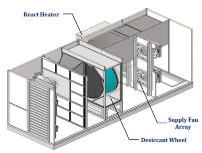
Desiccant dehumidification systems offer an effective solution to any application requiring room dewpoint temperatures below 50°F.
